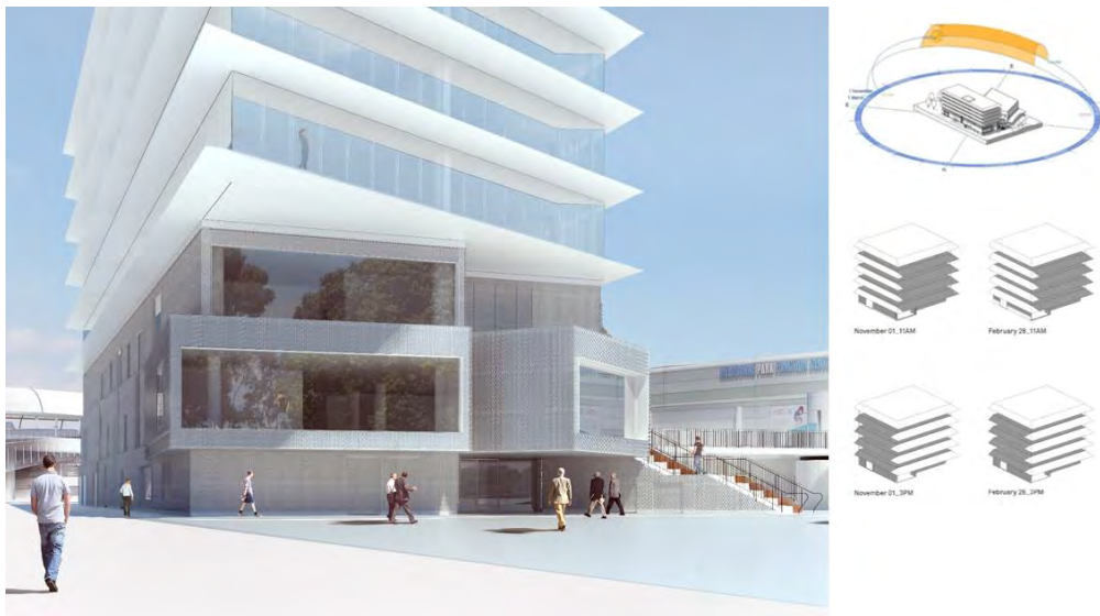
Image 04: Sunshading devices designed in Revit/Dynamo- Melbourne Park Administration and Media Building
